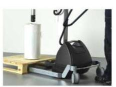
On several models, the measures of the wheels make it possible to drive the lifter into a Euro-pallet in three different ways.
