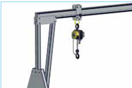
22. If the hoist is not already attached to the suspension point on the trolley, do so now (using stepladder if height setting requires).
