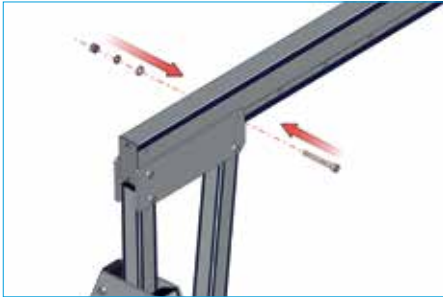
20. Insert and tighten the final beam bolt.
