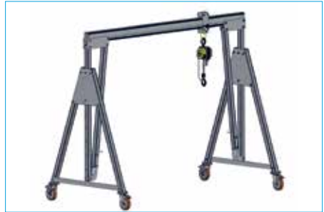
21. The gantry is now erect at its lowest height setting.
